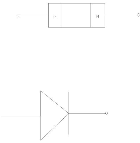
Junction diode is a solid state two terminal device which conducts with zero resistance when
