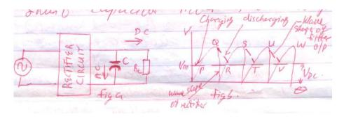
A large value electrolytic capacitor is connected is shunt (parallel) with the load RL as shown in fig a. the capacitors allow A. C. component of the rectified output to pass through it whereas DC component go straight to the load.
