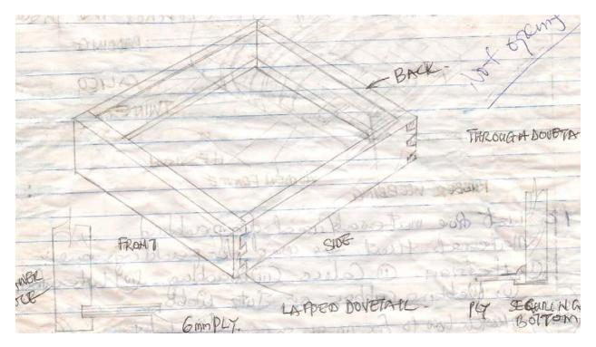
5b. The process of constructing a drawer with lap and through dovetail joint.
