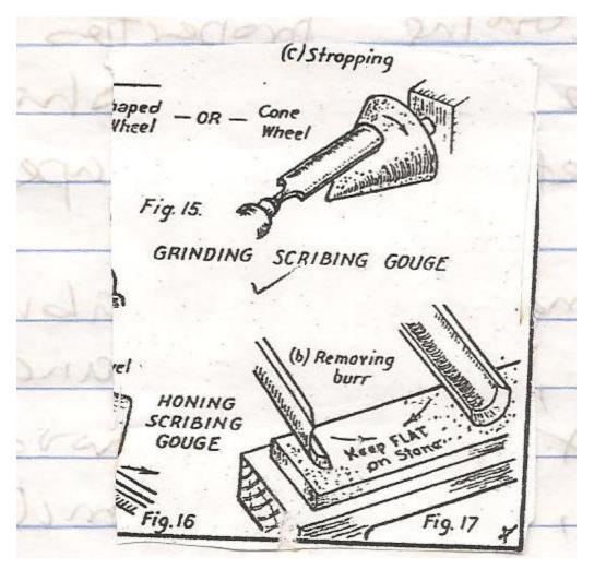
Uses: - It is used for contour work where hollow or concave curves are required.
