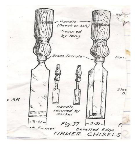
Uses: For general chiseling purposes. Being fairly strongly made it can be used for light chiseling with a mallet.
