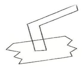
3. Bending: bending a straight rod in a hardy hole
