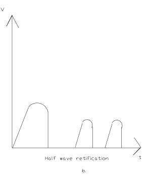
When the A.C. supply is on, electrons are drawn across the valve only on those halves of the secondary voltage cycles when the anode is positive.
