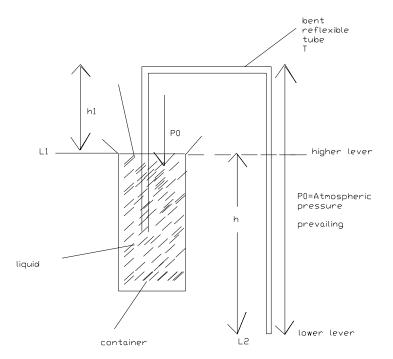
The siphon is a device for emptying containers which can not be easily emptied by tipping over. E.g. Petrol from a car tank or kerosene from a keg/jerry can.
