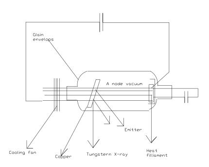
X-rays are produced when electrons liberated from a hot filament (thermonic emission) are accelerated through a high potential difference and are made to impinge on a metal target like tungsten.
