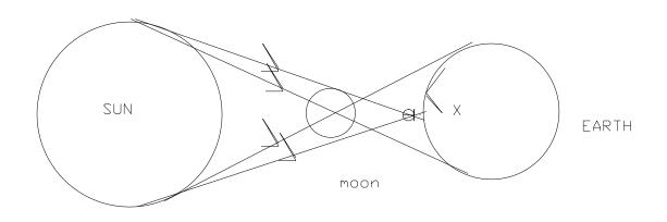
This occurs when the extreme rays at the moon's edge intersect before reaching the Earth as shown above. A ring of light is formed round the moon's shadow. The observer can be anywhere inside the region X on the Earth.
