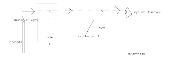
A small hole is punched in each of the cardboards A and b. They are placed in a straight line together with a light source. An observer is situated on the other side B. it will be found that the observer can only see light if the cardboards are well aligned. Light will pass through both holes.
