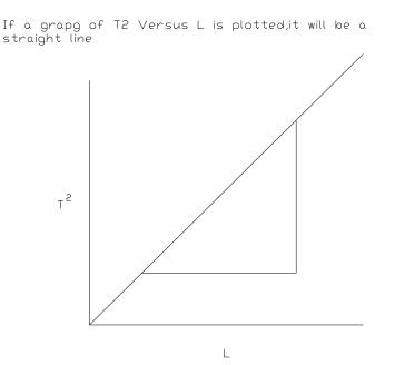
The shape of the graph  $S = (4\Pi^2)$ ; from which  $g = 4\Pi^2/s$ ; acceleration due to gravity at g the place the experiment was performed.
