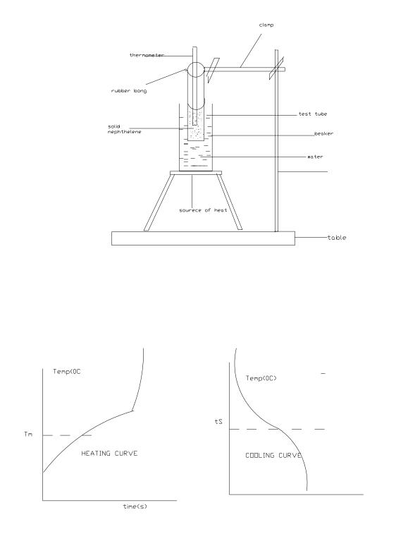
Precautions:- (1) Thermometer must always be in the midst of the Nephthalene. (2) Nephthalene must be of the highest purity (3) prevent parallax error in reading thermometer. Question 3(c) An iron of mass 5kg is heated to  $300^{\circ}$ C and is then quickly transferred to a block of mass 1kg at  $-2^{\circ}$ C. Neglecting heat losses to the surrounding, calculate the equilibrium temperature attained. Specific heat capacity of iron = 500J/kgk
