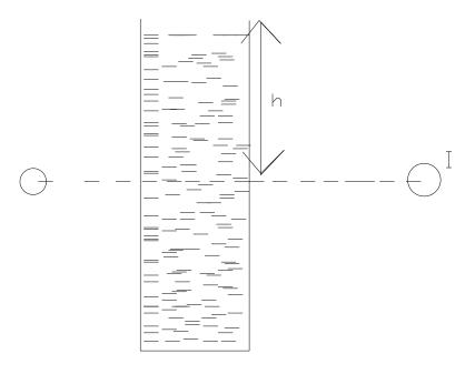
We want the pressure at the depth 00, pressure =  $\frac{\text{force}}{\text{Area cross section}}$
