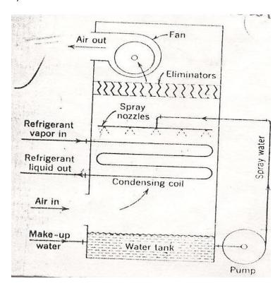
An evaporative condenser is essentially a water conservation device and is in effect a condenser and a cooling tower combined in a single unit and shown in the diagram below.
